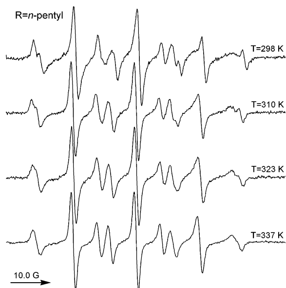
Figure 2. EPR spectra of nitroxide 6 recorded in the presence of MPC-C8-TEG 0.3 mM at different temperatures.
